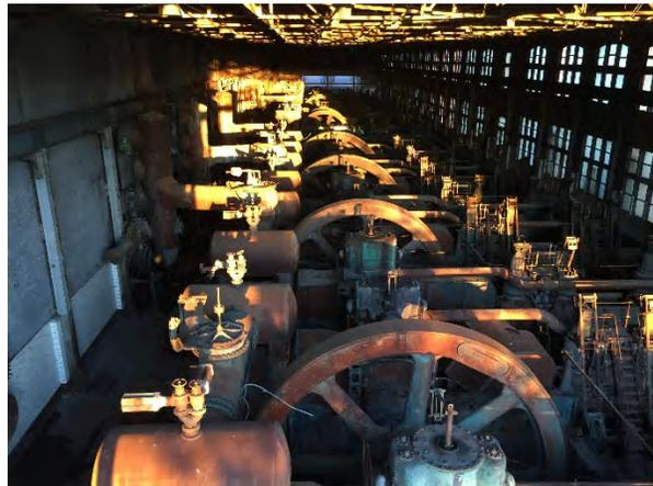
A view of the compressors inside the Blower Building. They supplied the air blast for the furnaces.
