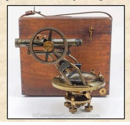
The transit was made to his order to accomplish the surveying work required to build the 15,000 foot-long Jeddo Mine Drainage Tunnel, which was built by McNair and his boss, John Markle (A.I.M.E. Honorary Membership in 1929.)
