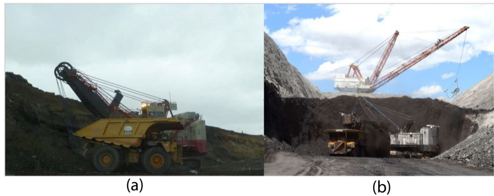
Fig. 3 (a) Truck and shovel excavating overburden Source: Photo by Amy McBrayer, (b) Dragline excavating overburden above truck and shovel loading Source: Photo courtesy of Wyoming Mining Association [24, 25]
