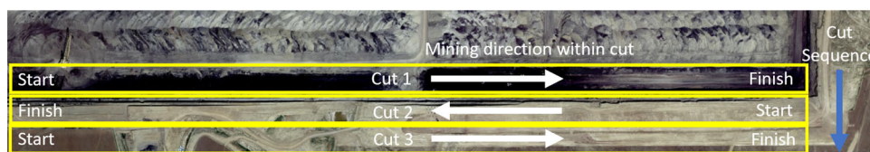
Fig. 14 Layover dragline pattern with dragline sequence for single pass mining. White arrows depict the dragline's mining direction within the cut and the blue arrow indicates the extraction sequence of the cuts. The
