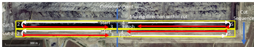
Fig. 15 Figure-8 dragline pattern in plan view with dragline sequence for two pass mining. White arrows depict the dragline's mining direction for the first pass within the cut while red arrows depict the mining direction for the second pass and the blue arrow indicates the cut extrac-
