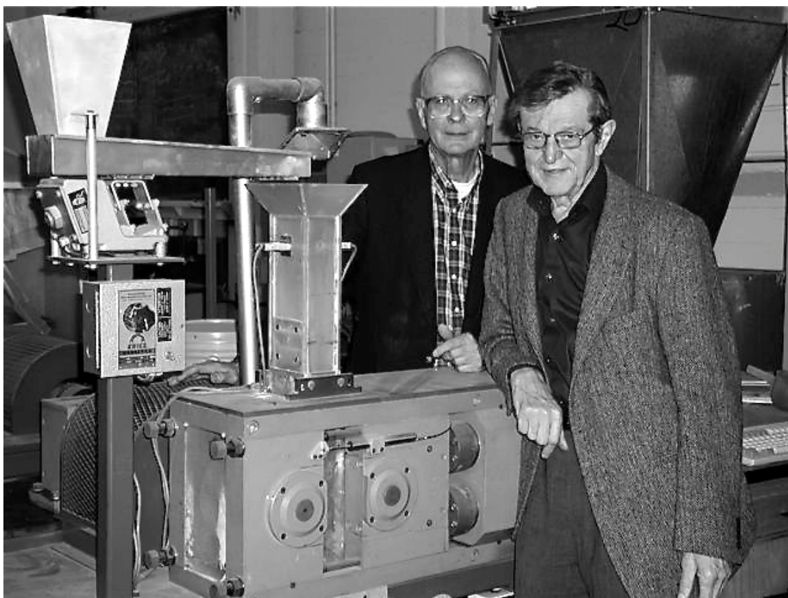
Photograph (2003) of Klaus Schoenert and DWF with the Clausthal-Berkeley laboratory-scale high-pressure roll mill (now being more generally referred to as high-pressure grinding rolls, HPGR). The counter-rotating rolls and their gear drive were manufactured in Schoenert's Institute at the Technical University of Clausthal, Germany, with rest being constructed and assembled in Berkeley.
