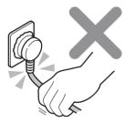
**DO NOT** damage the power cord and plug. Inspect both before installation to ensure all is intact.
