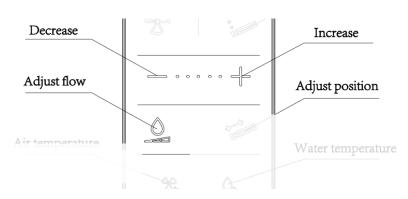
During the washing process, press the 'Adjust flow' button on the remote control to either decrease or increase the wash flow rate.
