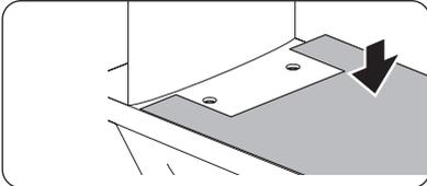
2. Place the installation template. Place the mounting template on the ceramic as shown. Align it with the rim of toilet.
