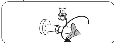
3B. Open angle valve to check for water leakage.
