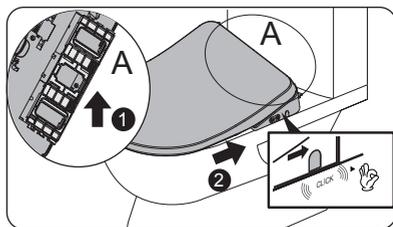
5. Slightly push the electronic cover plate into the fixing plate in the specified direction until the "click" sound is heard, indicating that the cover plate has been installed in place.
