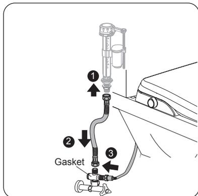
2A. After the filter and rubber gasket on both ends of the water inlet hose, connect the three-way joint with the cover plate.
