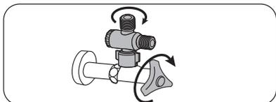
1A. Close the angle valve and remove the water supply hose connected to the water tank. The three-way joint is connected to the angle valve and ensure that the rubber sealing ring is loaded in.
