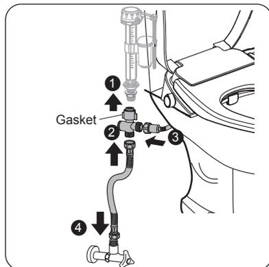
2B. According to the chart, after the filter and rubber gasket on both ends of the water inlet hose, connect the three-way joint with the cover plate.
