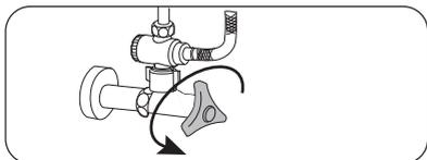
3A. Open angle valve to check for water leakage.
