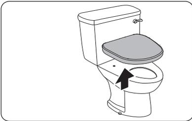
1. Remove the old cover plate. Loosen the nut connecting and move out the cover.
