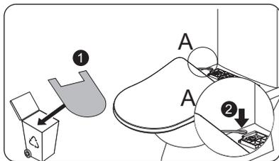
4. The installation template is disposable and recyclable. Please do not throw it away after installation. Then insert the inlet hose into the ceramic hole.
