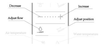
During the washing process, press the 'Adjust flow' button on the remote control to either decrease or increase the wash flow rate.
