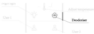
Repeatedly press the 'Deodorisation' button on the remote control to switch on or turn off the deodorisation function.
