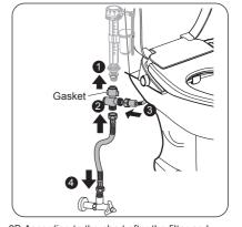
2B.According to the chart, after the filter and rubber gasket on both ends of the water inlet hose, connect the three-way joint with the cover plate.
