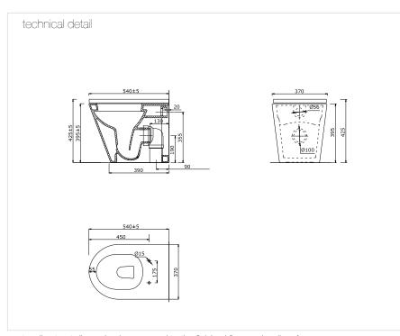
note: all set out dimension is measured to the finished floor and wall surfaces
