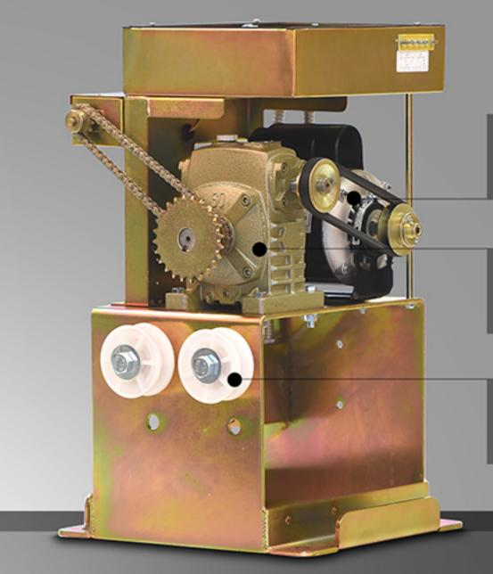
Continuous duty ½ and 1 horsepower models
