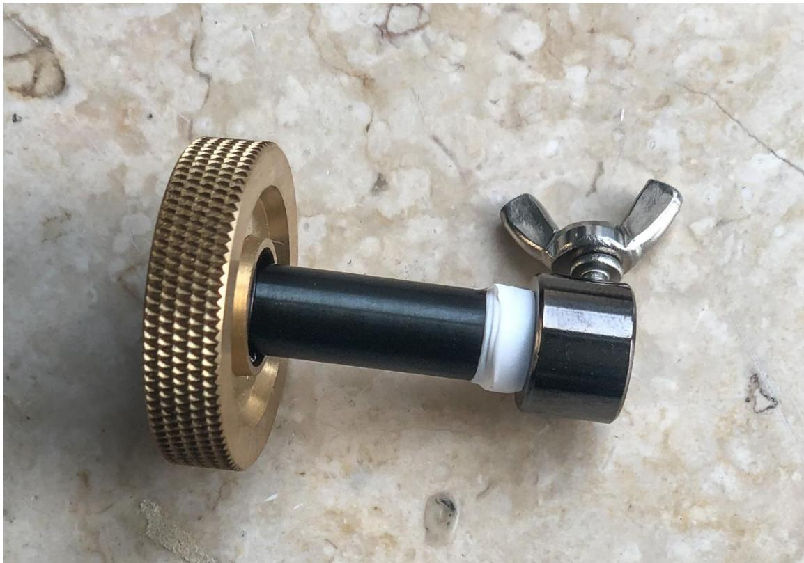
Be sure to thread a few turns of the Ball End Rod into the Collar. However, it is not necessary to completely thread it until it “bottoms out”. Just be sure there is enough engagement so that the assembly is secure.
