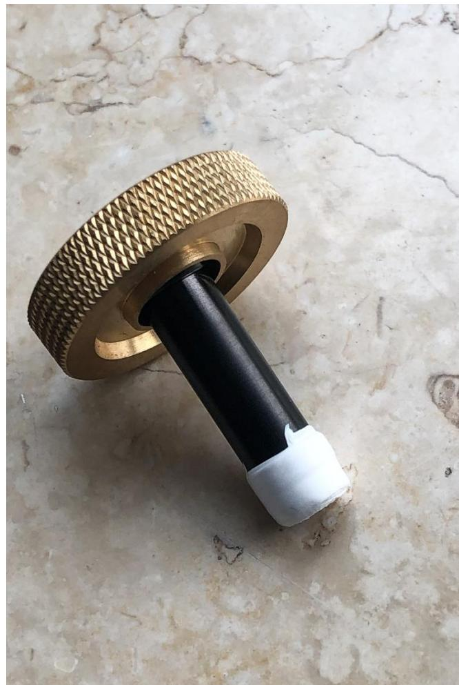
Step 4 – Thread the Collar back onto the Ball End Rod. Be sure you put the Retaining Cup (the big brass part) back in place correctly before putting the Collar back onto the Ball End Rod.
