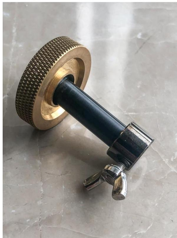
Step 2 – Unscrew the Collar from the Ball End Rod.
