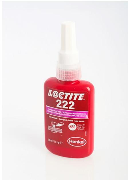
This is the mildest thread locker made by LocTite, and it may be possible to undo this if necessary. You may have better results, in case there is a need to undo the threading, by heating up the parts before attempting to unthread them.
