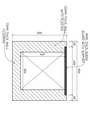
NOTE:ALL THE INTERNAL SURFACE TO BE APPLIED WITH WATERPROOF COATING. WATERPROOF COATING TO BE APPROVED BY CLIENT BEFORE APPLYING.
