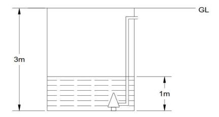
NPSH<sub>A</sub> depends on the particular pipeline system
