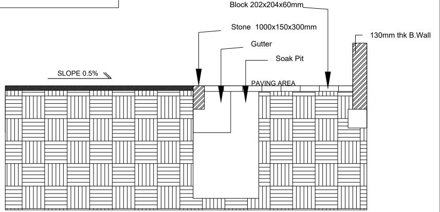
CURB STONE AND PAVING AREA SECTION DETAIL
