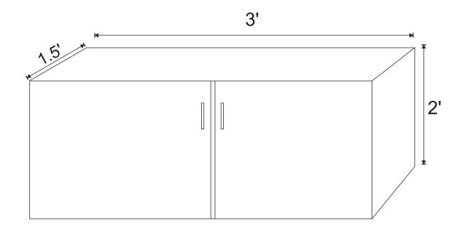
Cupboard ply wood 18mm (white) 2 cupboard hing Top granite sheet 18mm SS Sink 14"x 14" SS elbow tap
