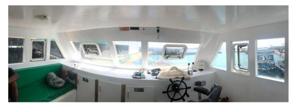
2- Enlargement of 03 cells in front of wheelhouse as per drawing (5FT x 3FT = 2NOS and  $20.5INCH \times 3FT = 1NOS$ ).
