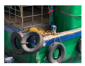
8- Install an appropriate rubber fender outside the front of the boat.
