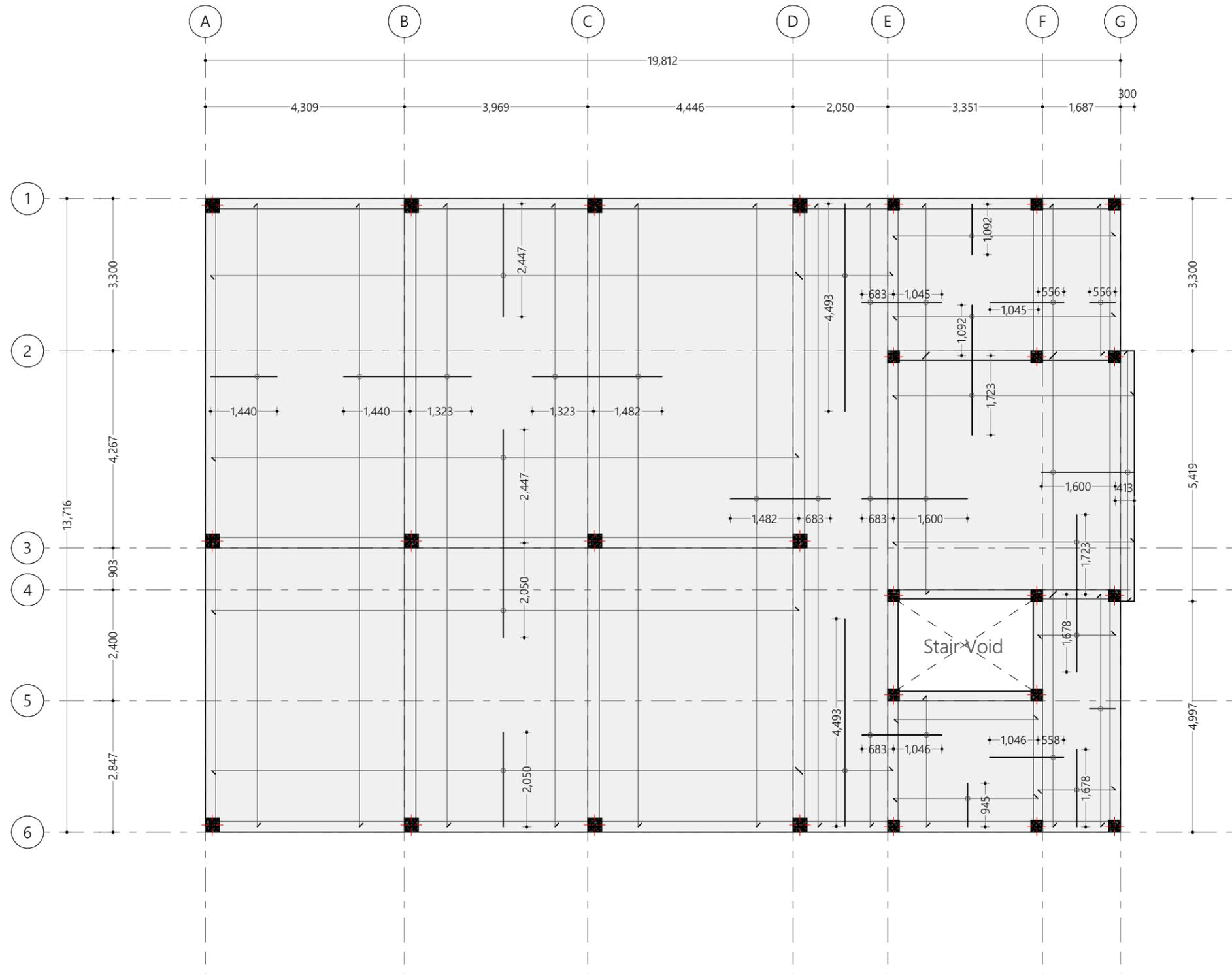
**Terrace Floor Slab Reinforcement Plan**
