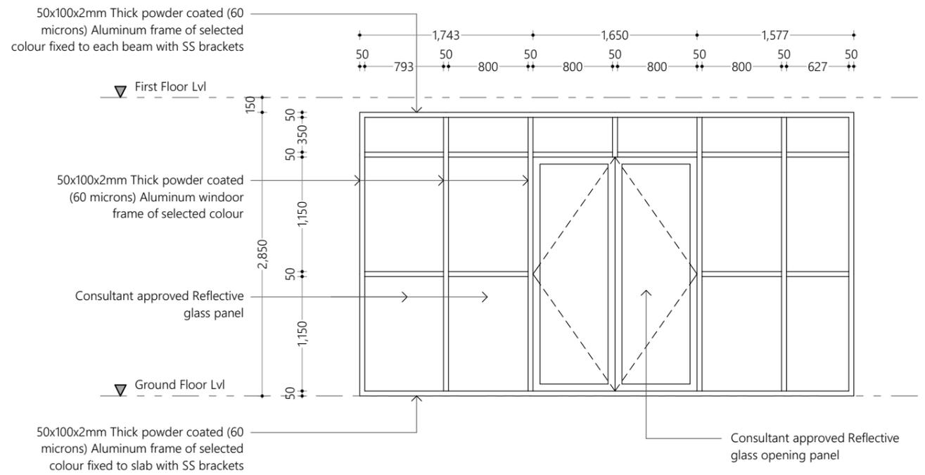
**Curtain Wall CW1 Detail - Elevation E1**
