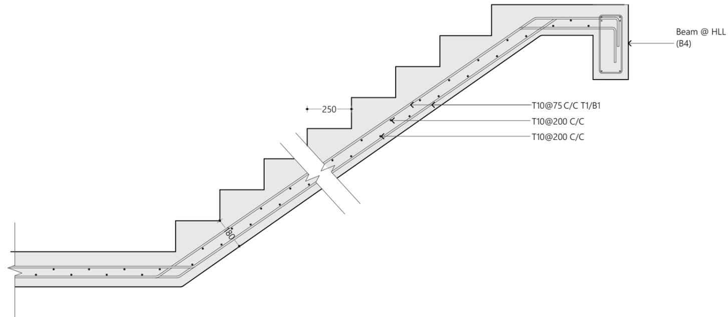
Staircase Reinforcement Detail
