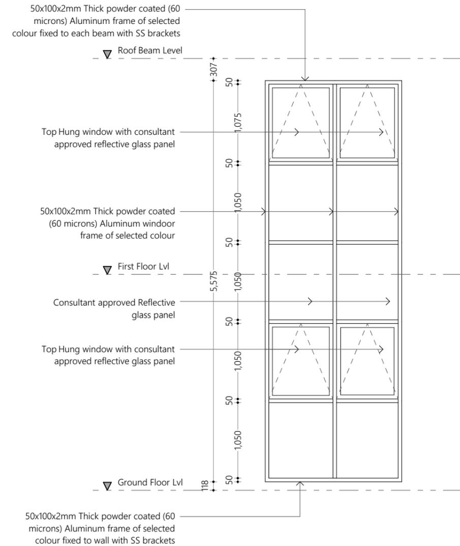
Curtain Wall CW4 Detail - Elevation E1 1:50
