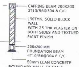
BOUNDARY WALL DETAILS SCALE 1:50
