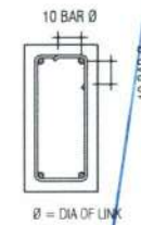
SHEAR LINKS ANCHORAGE DETAIL NTS
