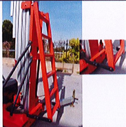
Insert aluminum support legs with rubber foot pad
