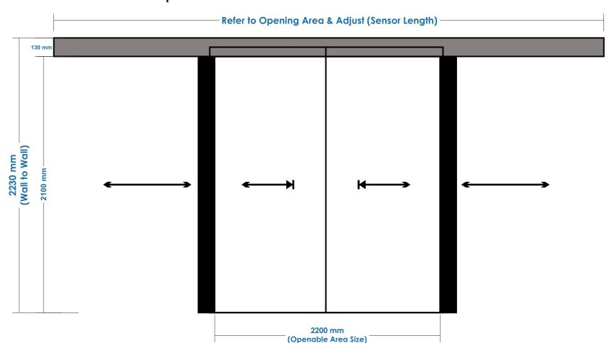
Automatic Sliding Sensor Door w/ Access Card Control System From Outside & Inside 12mm Clear Tempered Glass
