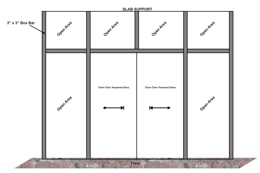
Automatic Sliding Sensor Door w/ Frameless 12mm Clear Tempered Glass.
