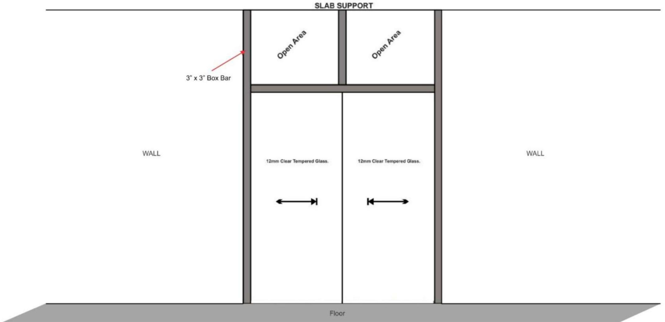
**Automatic Sliding Sensor Door w/ Push Button From Outside & Inside
