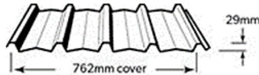
Figure 18: Typical Trapezoidal Roof Sheet
