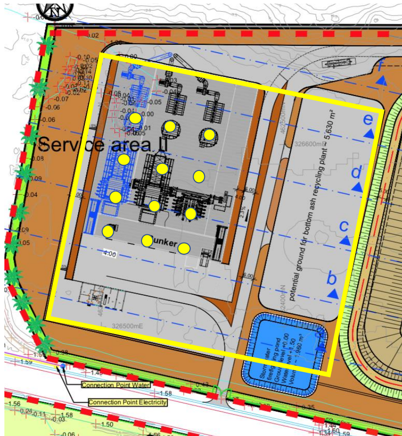
Figure 1: Test area plot on Thilafushi Island for geotechnical survey
