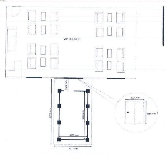
WALLS TO BE DEMOLISHED AND GLASS PANEL REMOVED
