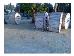
(Outer cover of cable drum must be properly packed and covered as per above picture)
