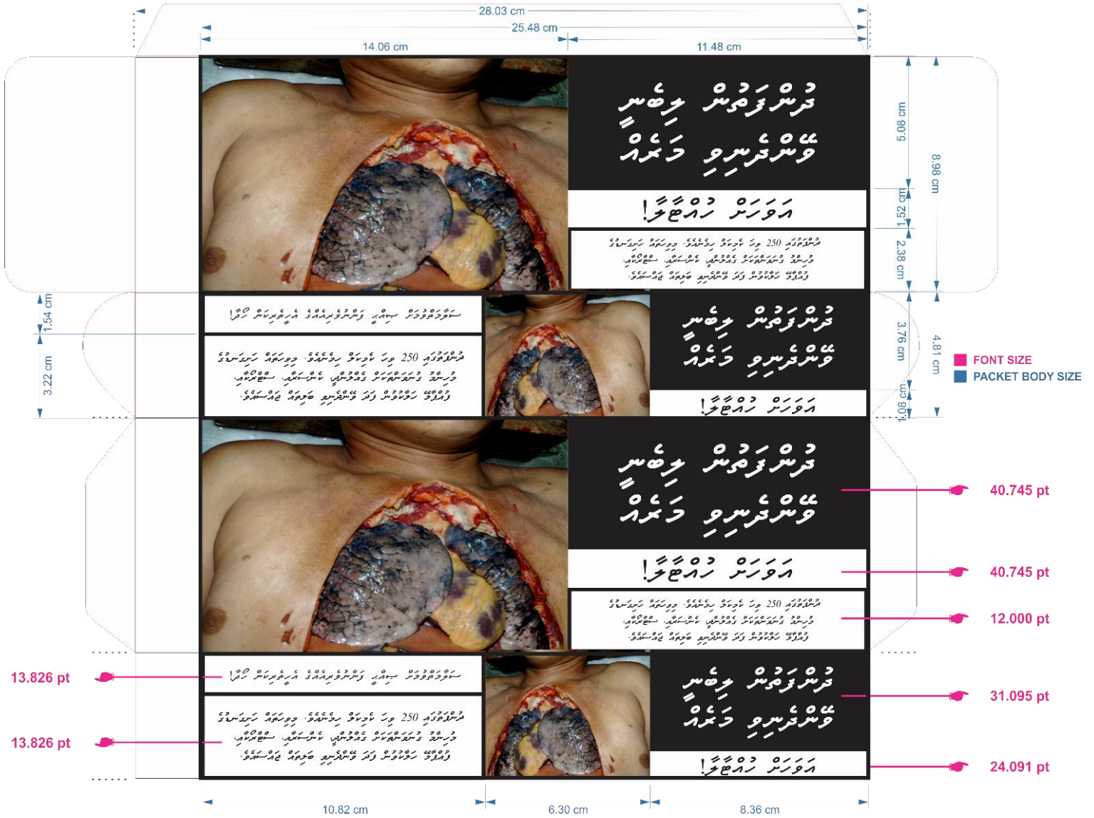
Exhibit-17: This illustration shows indicative sizes for various elements of the combined health warning for cigarette or similar carton
