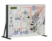
without a PC, guided by experimental book using built in oscilloscope or an external oscilloscope. The Simulator can be connected to a PC in USB communication using CBT courseware and D-SCOPE software for signal display. A record of the student progress can be recorded on the student PC using the optional DCML software and can be accessed by the instructor for monitoring, course management and records if a local area network (not supplied) is available.
