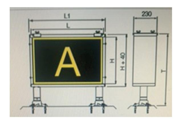
L = not less than 1100 mm L1 = 1148 mm Qty of Lamps = 2 nos H = not less than 800 mm Symbol Height = H/2 T = not less than 1020 mm
