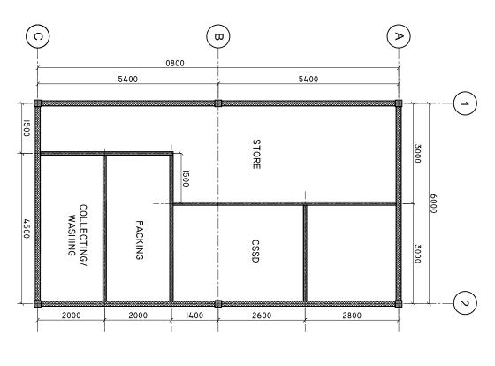
I50MM THICK HOLLOW BLOCK MASONRY WALL 125MM THICK DRYWALL PARTITION
