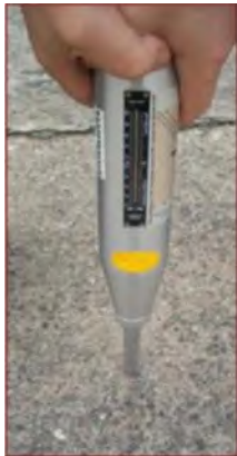
Compressive Test by Schmidt-Hammer test
