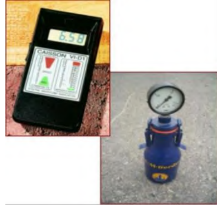
Moisture Test by Impedance
