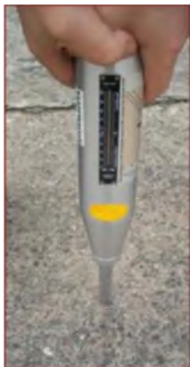
Compressive Test by Schmidt-Hammer test
