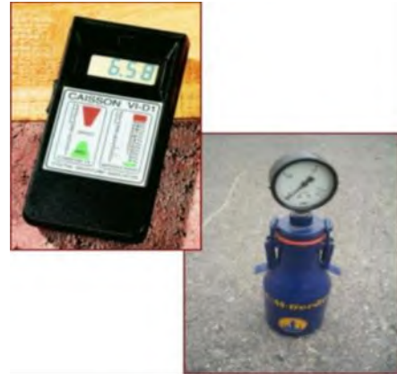
Moisture Test by Impedance
