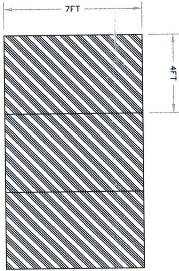
75MM THICK CONCRETE BLOCK
