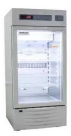
External size (W\*D\*H) mm: 500\*550\*1300 Capacity: 130L Temp. Range: 2°C~8°C Temp. Accuracy: 0.1°C Control system: Microprocessor control, large screen LED display Alarm: Audible and visual alarm for: High and low temperature, Power failure alarm, Sensor failure, Door ajar Refrigeration Type: Forced air refrigeration system Refrigerant: R600a, CFC Free Condenser & Evaporator: Bundy tube condenser Defrost: Auto defrost Door: Glass door with heat reflection film Shelves: 4pcs
