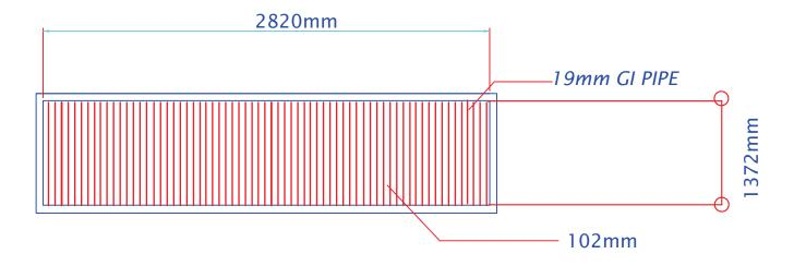
Total number of blocks to reinforce: 36 Distance between each pipe: 102mm (center to center)
