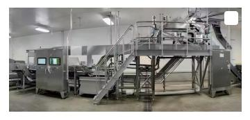
A fully automated sorter separates the nuggets, using high-precision laser imaging and computer vision algorithms to inspect and sort each piece to the processor's specifications.
