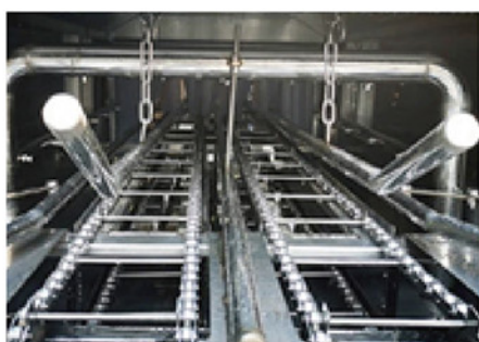
不锈钢输送链条 不锈钢链条/减噪耐磨/自动出料 Stainless steel conveyor chain, stainless steel chain/noise reduction wear resistance/automatic discharge
