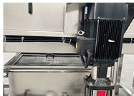
立式多级离心泵 扬程远/压力大/清洗效果好 Vertical multistage centrifugal pump, high lift/high pressure/good cleaning effect
