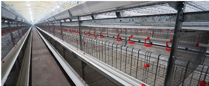
可伸缩式匀料器，克服因地面不平带来的落料不均。 The retractable feed distributor can overcome the uneven feed drop caused by uneven floor.
