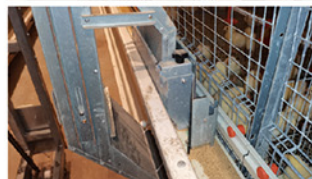
可伸缩式匀料器，克服因地面不平带来的落料不均。 The retractable feed distributor can overcome the uneven feed drop caused by uneven floor.
