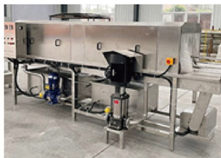
每段设有防水帘 保证每段清洗不相互交叉污染 Each section is provided with a waterproof curtain to ensure that each section is cleaned without cross-contamination
