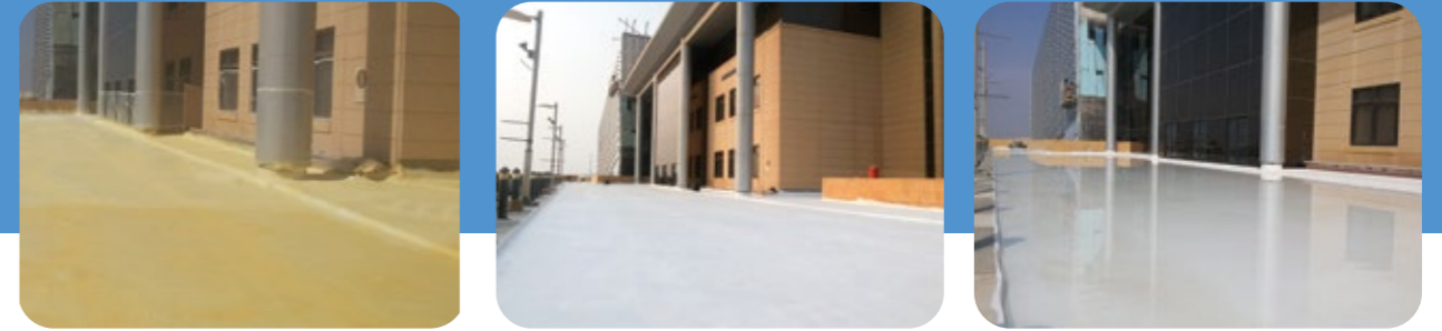
FLOOD WATER TESTING OF THE COMPLETED SYSTEM
