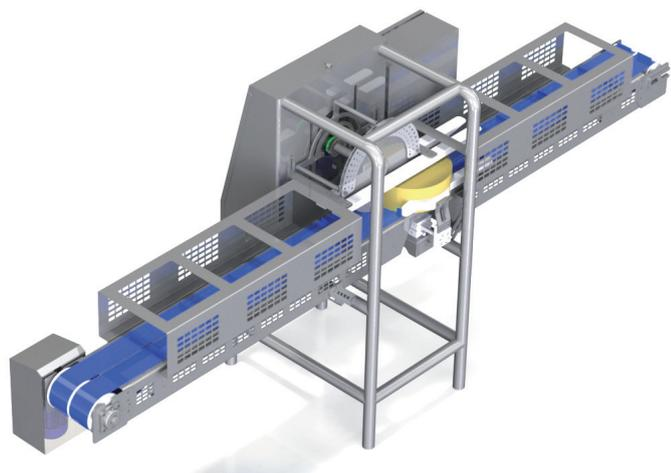
The system is ideal for cutting cheese blocks or round cheeses into halves. It is composed of a plastic modular conveyor belt for the infeed and outfeed of cheeses, and a tangential disc cutting unit. Specifically adaptable to different types, diameters and sizes of cheeses. Production: up to 750 cheeses/hour.
