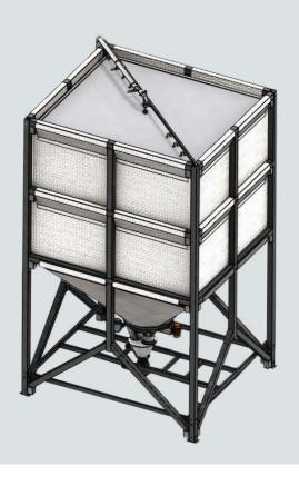
Reticular silos in high resistance Trevin fabric, for internal use. Equipped with a vibrating cone or fluidized bed extraction system, they allow the natural ventilation of the product; they have a reticular support structure, loading tube, integrated roof filter, maximum and minimum level probes, pressure switch, loading safety valve, pressure/Capacity: from 5 m³ to 100 m³.
