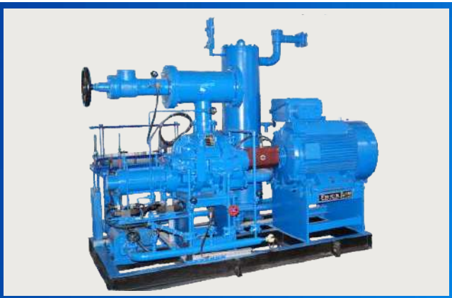
Frick India Rotary Twin Screw Compressor Package with Vertical oil Separator
