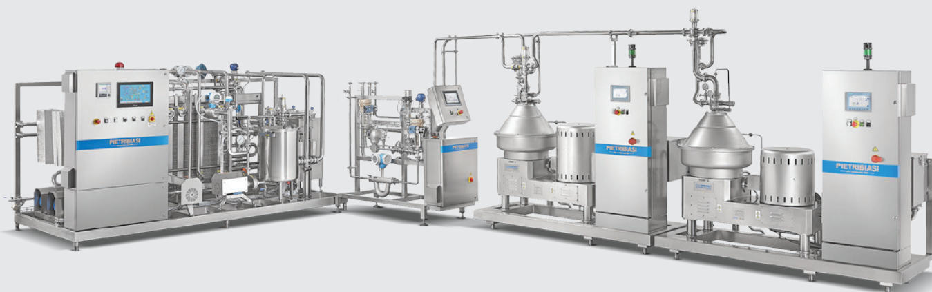
Pasteurization lines complete of bacteria clarifier, cream separator and automatic standardizer
