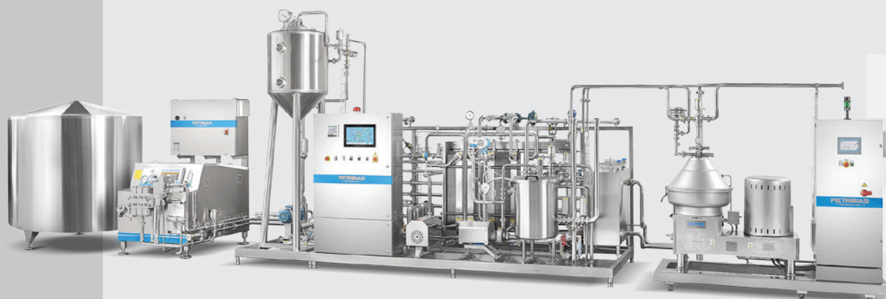
Customized pasteurization lines for cheese, fresh milk, fermented products, cream, full automatic version with CIP on board
