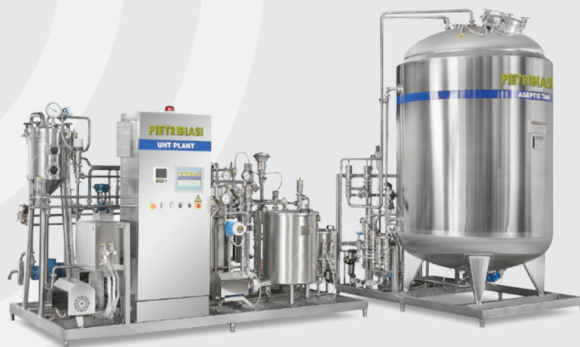
UHT plants complete of plate sterilizer, deodorizer, aseptic tank and sterile system
