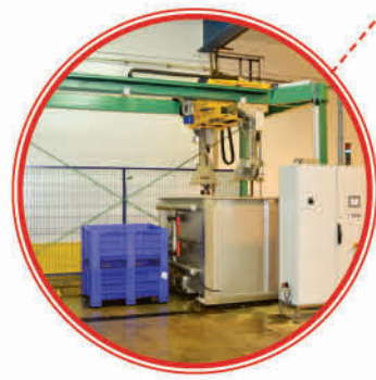
WET OR DRY AUTOMATIC BINS DUMPING SYSTEM
