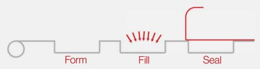
A Thermoforming vacuum packing machine combines thermoforming and vacuum sealing processes to create custom-shaped packaging for food. It removes air from the package to extend shelf life by reducing exposure to oxygen, preserving freshness and preventing spoilage.
