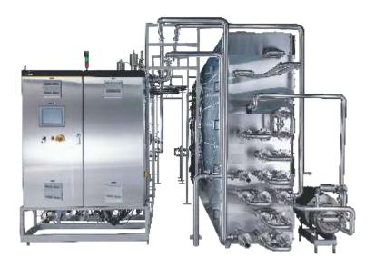
Designed and manufactured by Neologic Engineers, The UHT sterilizer module is tubular heat exchanger based, operating with variable speed to suit different flow rate. It features a system of heat recovery by a loop of sterile water. The tubular heat exchanger is a 'polytube' or shell and tube heat exchanger. It is rugged and flexible to suit sterilizing application with bellows.
