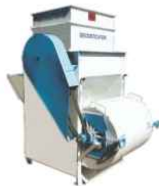
JATROPHA DECORTICATOR Capacity : 1 TPH - 5 TPH
