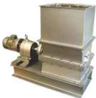
COPRA CUTTER Capacity : 500 Kg./Hr. - 5TPH
