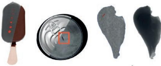
These systems include **complex algorithms** that provide the production line with a high capacity for **detecting all types of contaminants**. Varpe develops specific equipment for any product and sector. Additionally, they simultaneously verify damaged products, breakages, mass measurement and counting of elements within the product.
