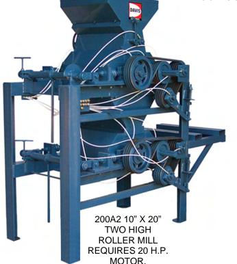
Ideal for feeding Poultry, Pork and Dairy, your target particle size can be achieved by adjusting the gap between the rolls. To adjust the gap the operator moves the lever attached to the eccentric shaft, which keeps the rolls parallel, and allows the rolls to be adjusted to within .006".
